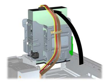
5. Rotate the power supply to its upright position. The hard drive is located beneath the power supply.
